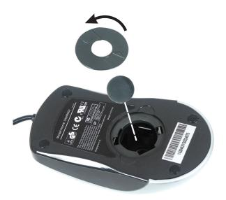
**3** Remove any dust, lint, or dirt from the mouse ball with a soft cloth.
